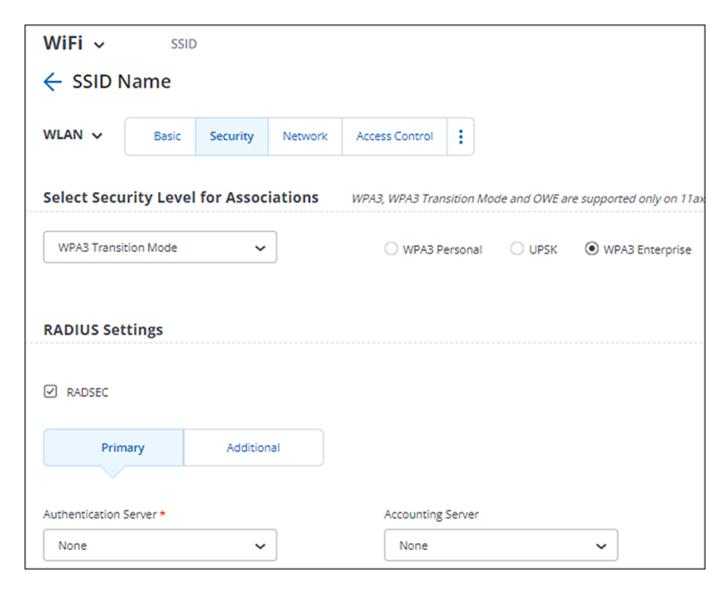
In the above screenshot, the RADSEC box is checked, so it is not vulnerable. If it is unchecked, then it is vulnerable.
